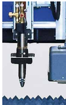
Stylus marker OmniScript Engraves characters, lines the part quickly and perm
