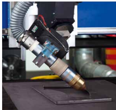
Plasma bevel cuts can be made quickly and easily with the Skew Delta.
